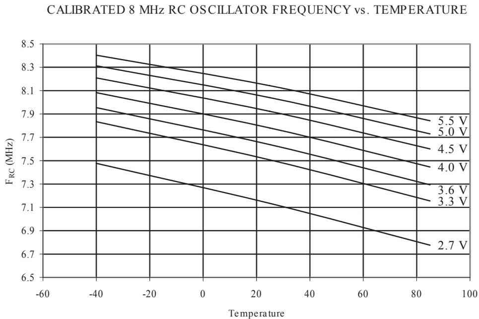
**Figure 31-36. Calibrated 8MHz RC Oscillator Frequency vs. VCC**
