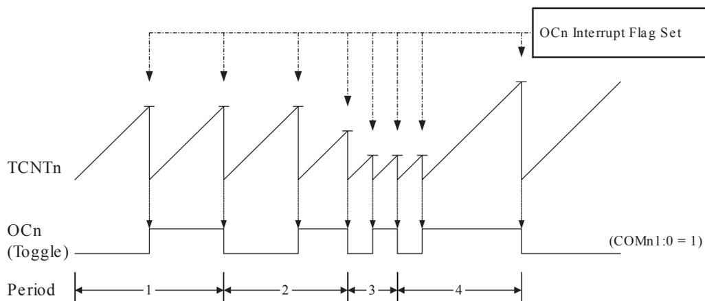
An interrupt can be generated each time the counter value reaches the TOP value by using the OCF0 Flag. If the interrupt is enabled, the interrupt handler routine can be used for updating the TOP value. However, changing the TOP to a value close to BOTTOM when the counter is running with none or a low prescaler value must be done with care since the CTC mode does not have the double buffering feature.
