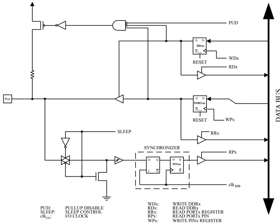
**Note:** 1. WPx, WDx, RRx, RPx, and RDx are common to all pins within the same port. clk<sub>I/O</sub>, SLEEP, and PUD are common to all ports
