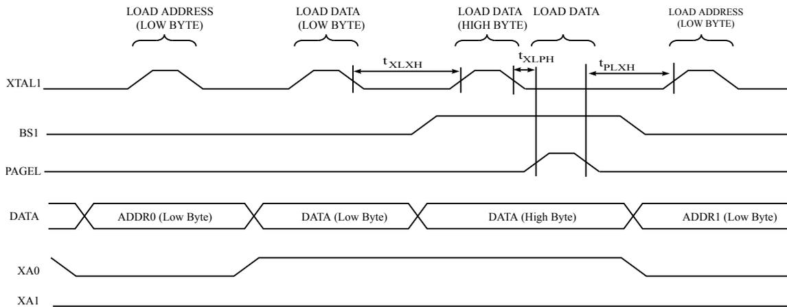
**Note:** 1. The timing requirements shown in the first figure in this section (i.e.,  $t_{DVXH}$ ,  $t_{XHXL}$ , and  $t_{XLDX}$ ) also apply to loading operation.
