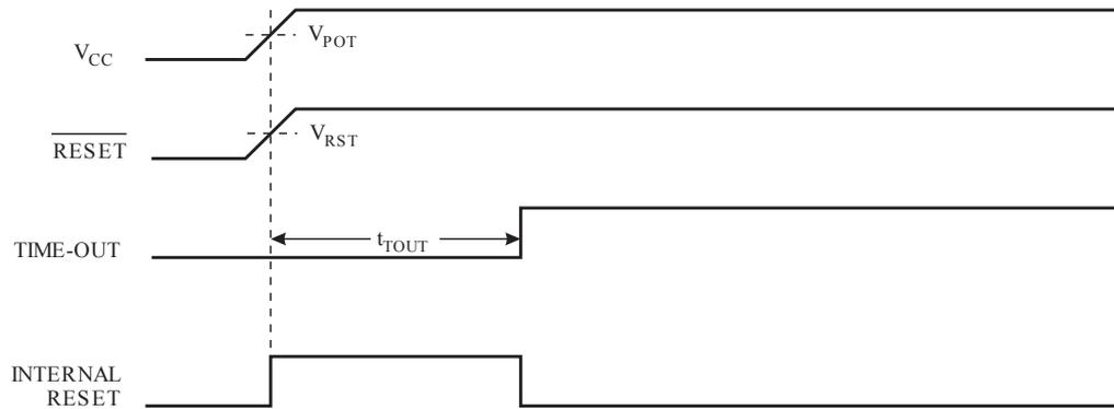
**Figure 14-3. Figure: MCU Start-up,  $\overline{\text{RESET}}$  Extended Externally**
