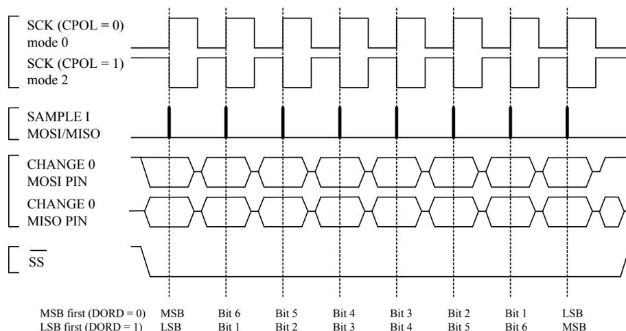
**Figure 22-4. SPI Transfer Format with CPHA = 1**
