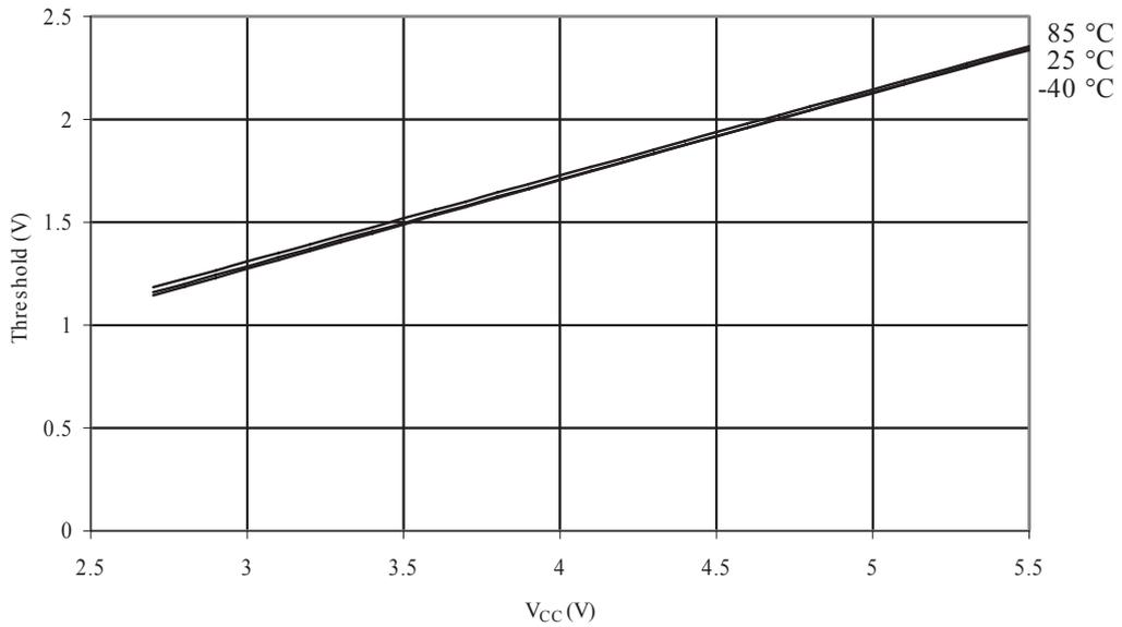
Figure 31-30. Reset Input Pin Hysteresis vs.  $V_{CC}$
